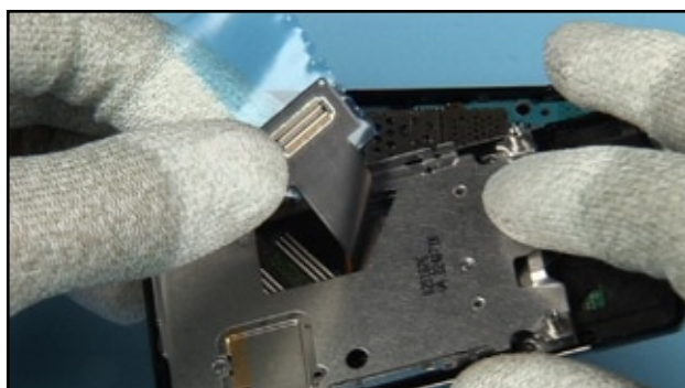
44. Carefully flip the flex foil as shown. Do not fold it!
